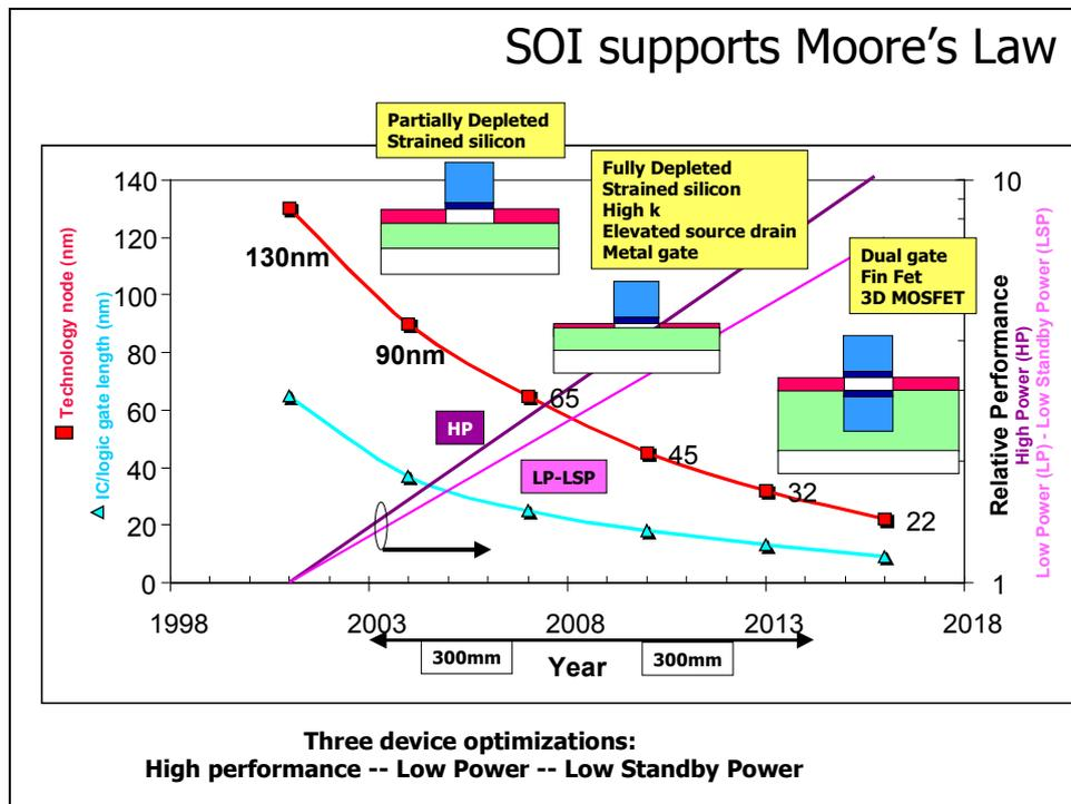
Figure 2. SOI fully supports future device generations
